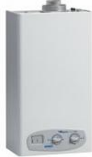
MORCO F11EL LPG WATER HEATER ROOM SEALED DIGITAL DISPLAY FITTED IN ANY LOCATION ELECTRONIC IGNITION W/OUT PILOT LIGHT CAN OPERATE ON LOW WATER PRESSURE & FLOW RATES FLUEING OPTIONS BOTH HORIZONTAL AND VERTICAL MAX CONSUMPTION 35W 12V SYSTEM WITH SMALL INVERTER FLUE AND FITTING KIT NOT INCLUDED NEW INSTALLS REQUIRE A (N240/KIT) FITTING KIT AND A FLUE KIT 330(W) X 230(D) X 595(W) N240 593.45
