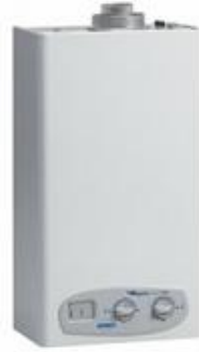
MORCO F11EL LPG WATER HEATER ROOM SEALED, FEATURES A DIGITAL DISPLAY, IT CAN BE FITTED IN VIRTUALLY ANY LOCATION, IT HAS FULL ELECTRONIC IGNITION W/OUT A PILOT LIGHT AND CAN OPERATE ON EXTREMELY LOW WATER PRESSURE AND FLOW RATES, FLUEING OPTIONS INCLUDE BOTH HORIZONTAL AND VERTICAL, MAX CONSUMPTION 35 WATTS, COULD BE USED ON A 12V SYSTEM WITH SMALL INVERTER, THE FLUE AND FITTING KIT NOT INCLUDED NEW INSTALLS REQUIRE A (N240/KIT) FITTING KIT AND A FLUE KIT 330(W) X 230(D) X 595(W) N240 593.45
