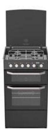
THETFORD CAPRICE 36I OVEN/GRILL Overall Dimensions 844 x 513 x 500 Build-In Dimensions 846 x 496 x 490 Total Heat Input 8.6kw GAS BURNERS 1 x 1.0 kW 3 x 1.5 kW IGNITION 12V GRILL BURNER 1.6 kW OVEN BURNER 1.8KW D430/B 619.00
