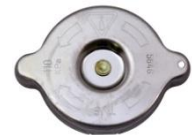
HEADER TANK CAP RDG1723 5.90
