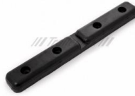
T4423 2.95 SNUBBER BLOCK 304mm LONG WITH 4 HOLES FOR 8 mm BOLTS CAN BE USED STRAIGHT OR AS V
